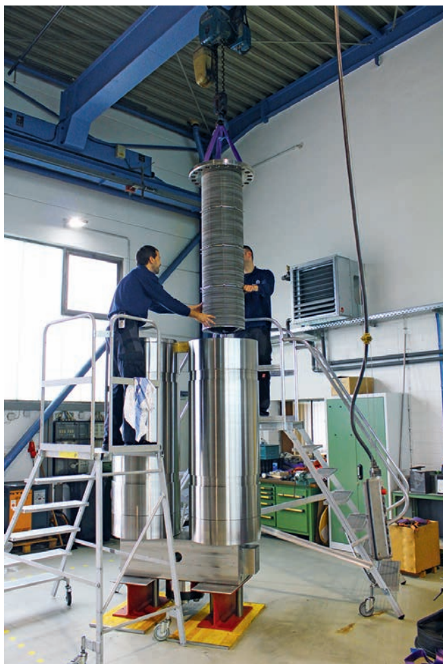
Fig. 1. Switch-over: this large surface filter can work continuous, as the operating team can switch between the filter disc stacks during operation
